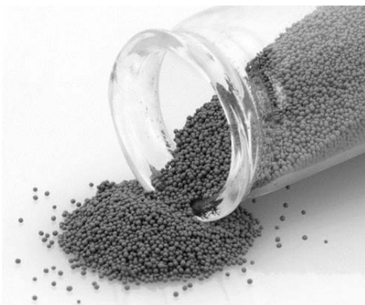
Left: CALORIVAC-H ® granules produced at VAC. Right: Typical adiabatic temperature change of the produced spherical particles
