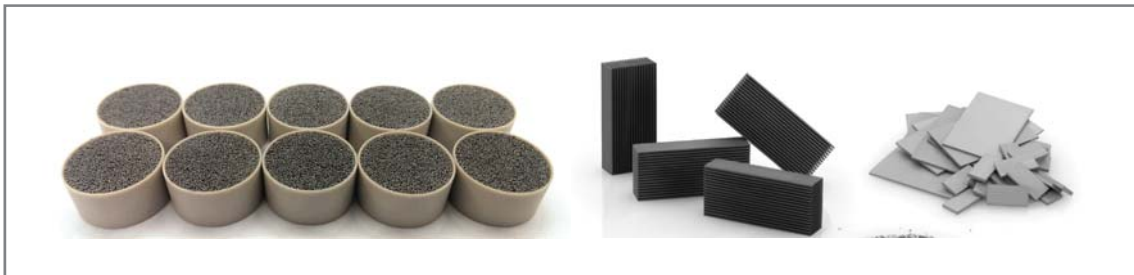
Example structures of La-Fe-Si based alloys. Left: Bonded spherical particles, Middle: Parallel plate structures, Right: Individual plates.
